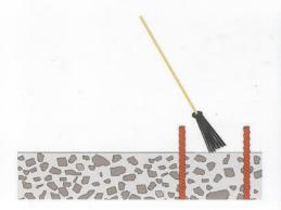
Clean surface from dust, dirt and loose particles.
