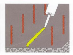
Apply adhesive to concrete or swelling gasket.
