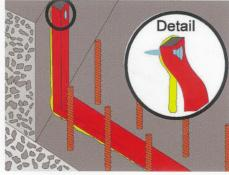
For vertical installation, apply swelling gasket with adhesive and use nail to hold until it dry. Remove nail after adhesive has set and cut away punctured gasket.
