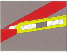
Cut the swelling gasket with knife to desired length.
