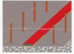
Butt joint for the connection of gaskets. Coverage min. 8 cm (3.15 inches)
